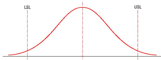
*Distribution curve of checks on incoming goods can indicate if the supplier is filtering out bad quality*
