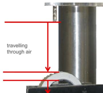
*Excessive distance travelling through the air is a process waste*
